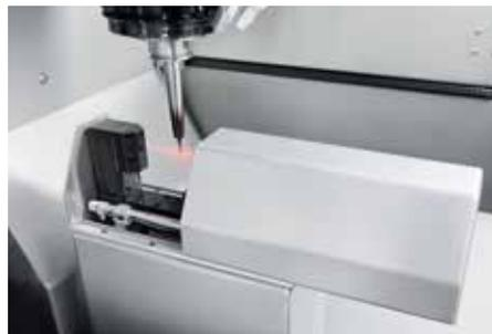
The fast tool change by means of a double gripper is a standard at exeron. The tool magazine offers space for 30, 60 or 90 tools.
