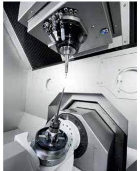
The laser enclosure prevents erroneous measurements linked to contamination and it is optionally available for the HSC MP7.
